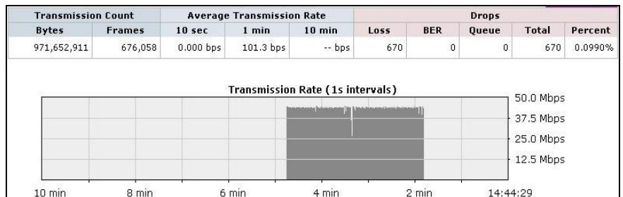
Figure 5 – 1 st Pass Performance. WANScaler 8800 transferring 900 Mbps of data over a 45 Mbps link with impairments. WANScaler completes the transfer in 3 min.
